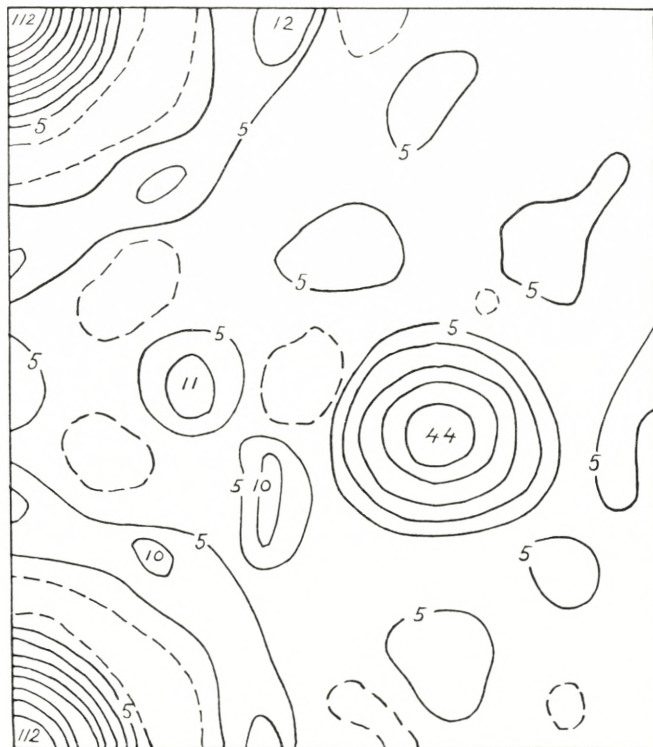
Fig. 6. Projection on 11\bar{2}0 plane from calculated F values for an arrangement of \text{SrCl}_2 with Sr at 000 , Cl at \frac{1}{3} \frac{2}{3} 0.42 and \frac{2}{3} \frac{1}{3} 0.58 .
