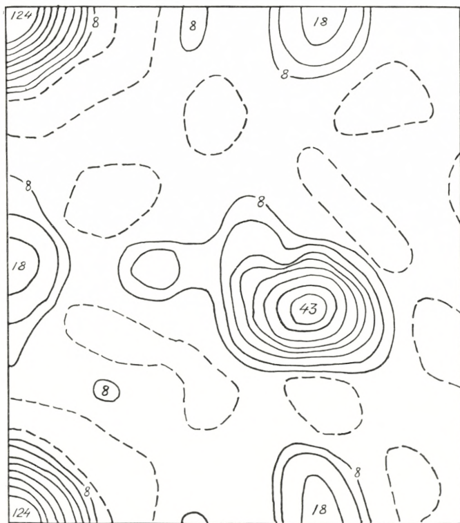
Fig. 8. Projection on 11\bar{2}0 plane in proposed arrangement of \text{SrCl}_2 \cdot 6 \text{H}_2\text{O} . From calculated F values.
